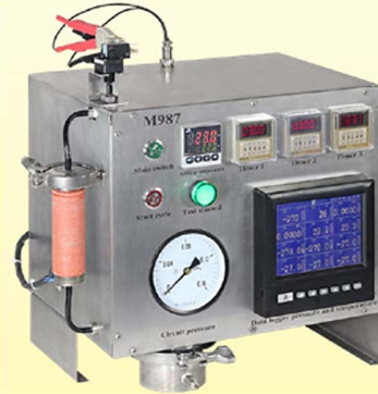
Test equipment for measuring, recording and setting the barometric and the ambient temperature compensation systems of the air switches (Ultimheat Laboratory)
