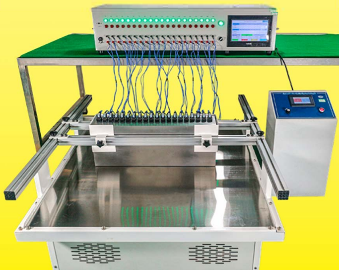
Test equipment to measure the vibration resistance of air switches and slow-action contact of pressure switches by simulation of transport conditions (Ultimheat Laboratory)
