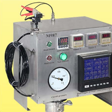
Test equipment for measuring repeatedly and constantly the maximum length of the air switch connecting tubes according to the volume of the push button and the pressure it develops (Ultimeat Laboratory)
