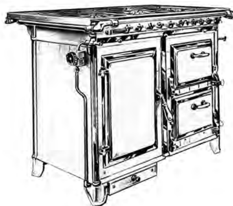
Model 506 cooker with "Telegaz" oven thermostat. The rod thermostat and the burner are independent. (Catalog 1932 Arthur Martin *)
