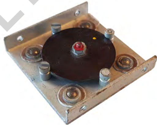
Top and bottom view, snap-action temperature limiter with 29mm disc used on military radio equipment to turn on ventilation. Type "Blower thermostat" (Around 1935-37, **)
