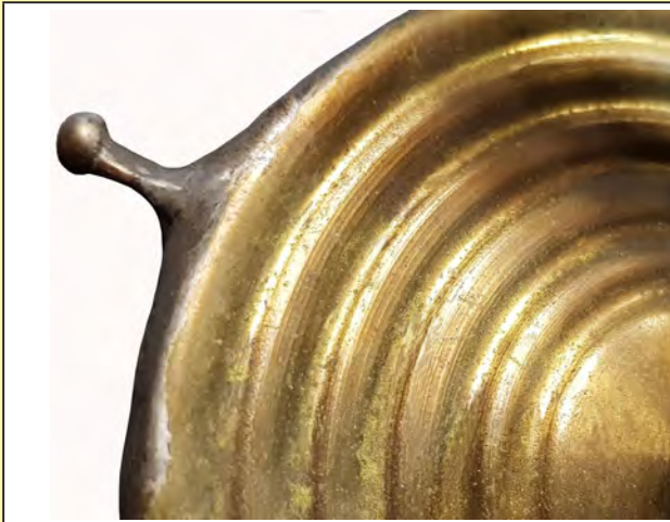
The corrugated membrane of one of Lucien Vidie's first aneroid barometers, traces of the embossing tool are visible, as well as the tin solder. (**)
