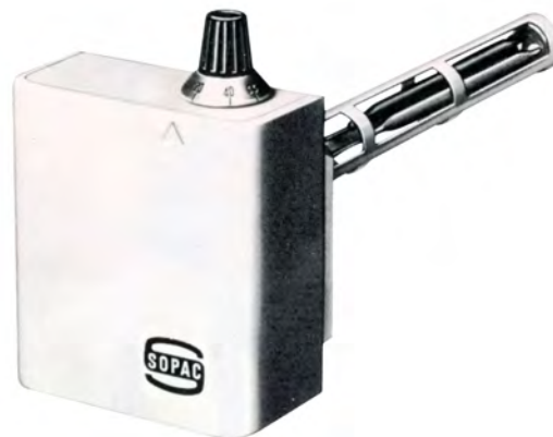
Airstat for forced air heating systems, two bulb liquid expansion mechanism for regulation and safety. Snap-action microswitch contacts. ST series (1977 Sopac Catalog *)
