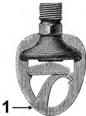
Grinnell fusible alloy sprinkler head of the first model on the market. In 1, solder with fusible alloy. (The Pantheon of Industry of February 22, 1885)
