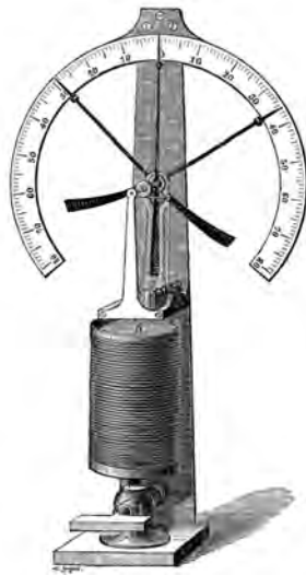
Lucien Vidie's corrugated tube pressure gauge (Biography of Lucien Vidie, by Auguste Laurent, 1867*)
