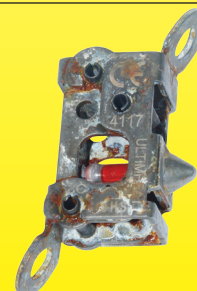
Zinc plated steel fire detection mechanism after 240h salt spray at 20%
