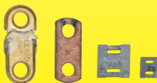
Copper, brass, and coated fusible links after 300h salt spray at 20%
