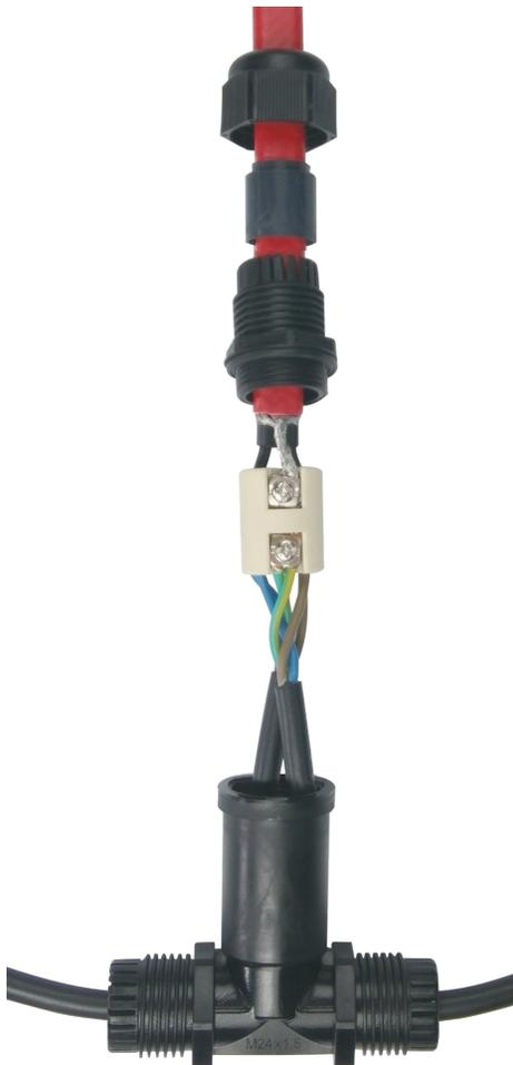
Slide the ceramic terminal block into the body, pushing it and simultaneously pulling on the round cables. Then screw the body of the cable gland A without having entered the flat cable silicone gasket.
