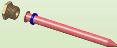
External diameter 8 mm, internal 6.5 mm, with flat seal bearing. Mounting with 1/4" BSPP brass nut and a flat internal fiber gasket (included). These cheap pockets (no solder nor brazing between the joint and the tube) are designed for dia. 6mm bulb or sensor insertion. They are not suitable for the pre-wired thermal cut-offs (see page 130). Putting some thermal compound on the sensors improves the response time. The kit includes: nut, pocket, fiber gasket.
