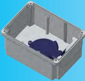
Powder painted aluminum housing base designed for rear mounting applications. Can receive threads from 3/8" up to M77 or 2" for thermostat rods or for immersion heaters. Allows to cover the whole range of these applications
