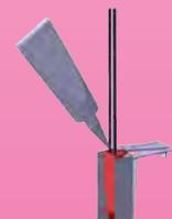
Fill with liquid silicone in the largest neck (connection wires outlet). It is possible to cut the insertion and filling flaps after polymerization.
