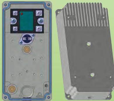
Part of the housing is provided for mounting a single-phase SSR, up to 25A rating, whose heat exchange is provided by cooling fins at the rear side. In this application, it is also possible to use the disc thermostat slot to install an overheating safety thermostat for the SSR
