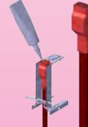
Position the assembly on the filling support and lock it with the upper flap of the sleeve, which has a flange for this purpose. Fill with liquid silicone in the upper shell-hole. It is possible to cut the insertion and filling flaps after polymerization if necessary.
