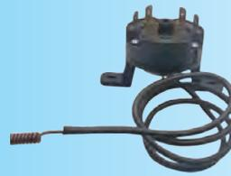
3 pole manual reset high limit manual reset thermostat, fail safe, fixed setting, temperature range up to 170°C
