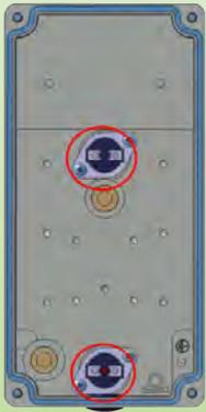
2 available slots for disc thermostats. They have extended cup brackets, for throw wall mounting to limit the thermal inertia in air heating systems devices. Safety or control applications. Disc thermostats: see page 130
