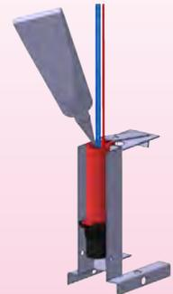
Position the assembly on the filling support and lock it with the upper flap of the sleeve, which has a flange for this purpose. Fill with liquid silicone. It is possible to cut the insertion and filling flaps after polymerization.
