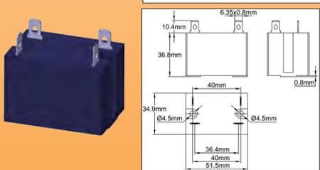
1 x 30A 250V resistive (AC1) (CE and UL) NO contact, sealed housing, 6.35 x 0.8 terminals. This relay can be mounted without mounting plate directly on all plastic triggered front provided for bulb and capillary thermostats and electronic controllers, and on the flat fronts of the distribution boxes in this catalog
