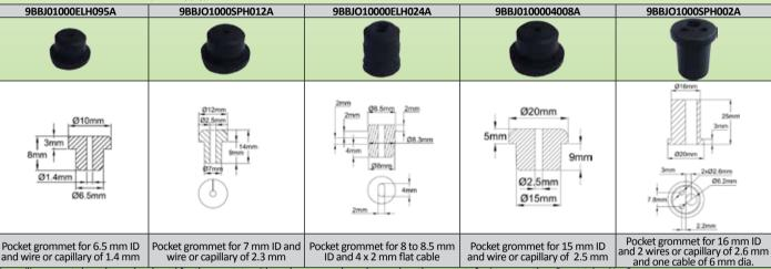
Many silicone parts have been developed for thermostats with enclosures, and can be used on thermostats for incorporation. See catalog No. 2
