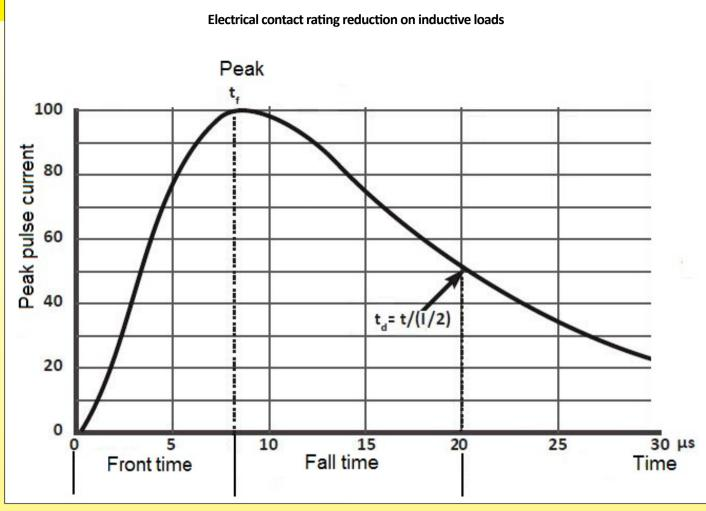
Overvoltage peak on inductive load circuits
