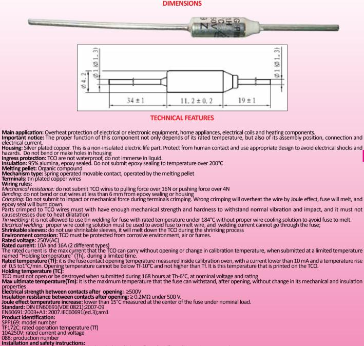
· Choose TCO temperature fuse which electrical insulation will not be effected by equipment overheat. TCO replacement must be made by exactly the same model of the same supplier
