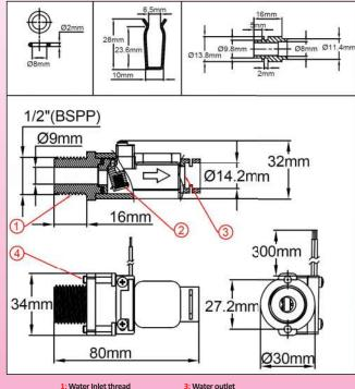
Main applications: Product developed for miniature instantaneous water heaters for showers. The mobile flap system provides compactness. Water inlet is done directly by the ½" BSPP male thread. Mandatory vertical mounting, with water inlet from the bottom. Connection to internal copper piping DN8 and DN10 with quick coupling
