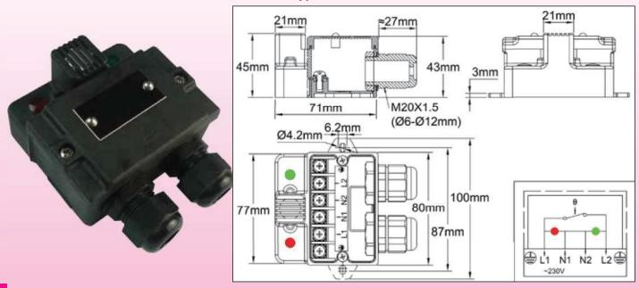
In these boxes, the thermostat, bimetal disc type, is over-molded, and is thermally insulated from the wall on which it is mounted. Its temperature sensing cup is mechanically protected by a grid. It is located in front of the enclosure to be in an area of natural circulation of air.
