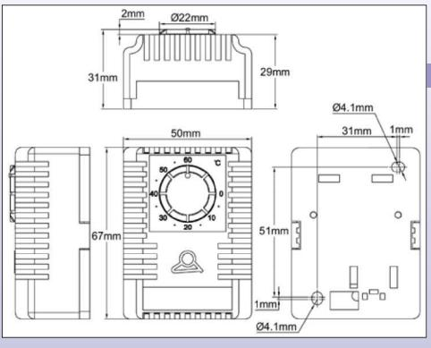
These models have been designed to control electrical equipment temperature. They are designed for wall mounting with 2 backside screws.
